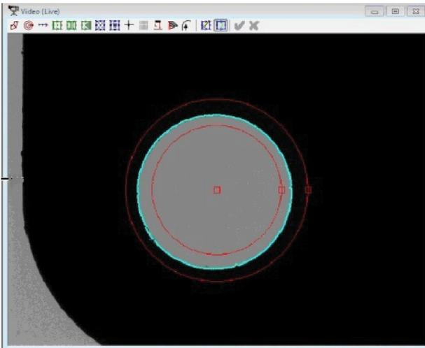
**Figure 1: Video Measurement of a Thru-Hole**
